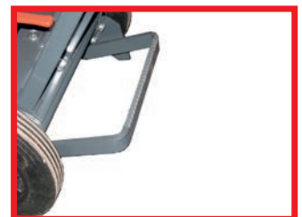
FOOT OPERATED DEPTH CONTROL
