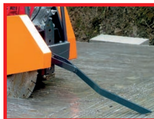
POINTER GUIDE FOR IMPROVED ACCURACY
