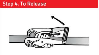
Pull the ratchet handle up to (180°) releasing the failsafe mechanism.
