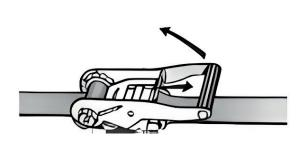
Pull the ratchet handle up to (180°) releasing the failsafe mechanism.
